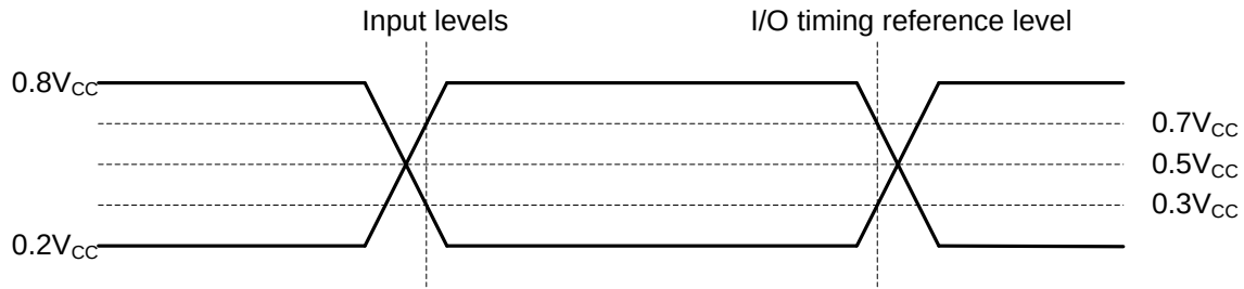
Figure 30: AC Measurement IO Waveform
